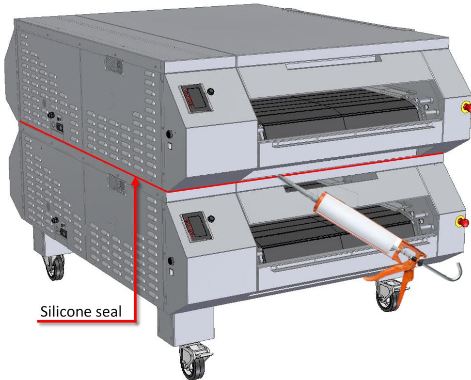
When stacking multiple ovens, a high temperature silicone must be applied between each unit to ensure a proper seal (shown in red). The seal must go all the way around the ovens with no gaps.
