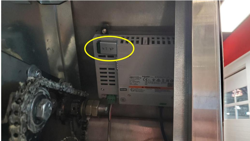
/ Accept the USB transfer on the HMI screen.
